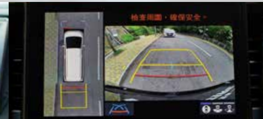
原廠360鏡頭及動態泊車輔助綫 Genuine 360-degree Camera with Dynamic Park Assist Lines
